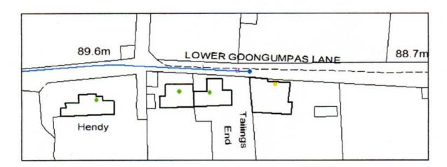
The stop tap for Mr Layte's supply is located at the side of Lower Goongumpas Lane and displayed on the photograph below. The location of the hydrant is also displayed in this photograph. The exact location of the communication pipe is not known but assumed to run from the water main to the stop tap. The pipe from the stop tap is Mr Layte's private supply pipe.
